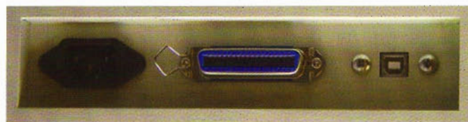
Figure 10: The GX can be driven using a traditional parallel port printer cable or a USB cable.
