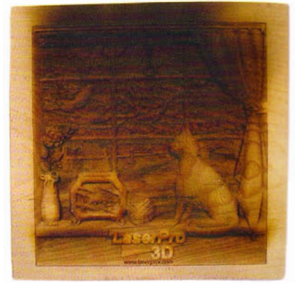
Figure 9: This first attempt at 3-D engraving wood is a reminder that 60 watts is a powerful laser.
